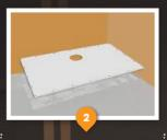
Excavate the floor within the marked area to a sufficient depth of 24mm to accept Tuffdeck.
